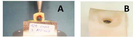
A: push-out set-up, B: no delamination of NCD
